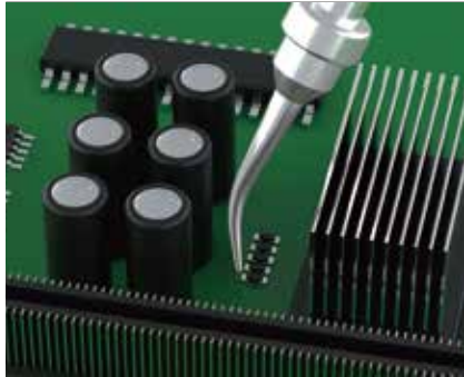
You can choose a soldering tip according to your needs, suitable for various soldering processes (Bent tip soldering iron tip, suitable for soldering in narrow spaces)
