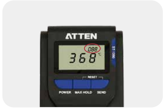
Display the number of temperature measurements and record the current usage of the sensor for easy determination of replacement cycles
