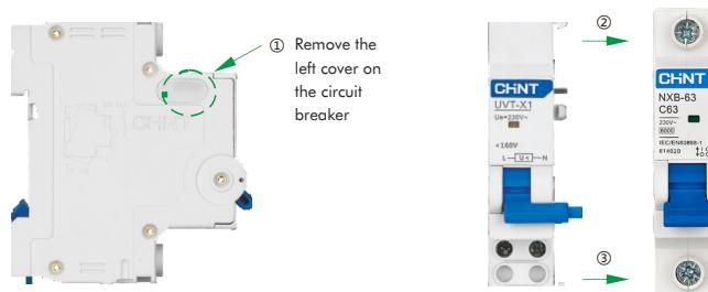
After the release is assembled with the circuit breaker, mount them on TH35-7.5 steel mounting rail.
