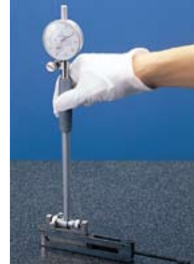
Setting a bore gage using a holder with the pair of Type I half-round jaws arranged as flat contact surfaces
