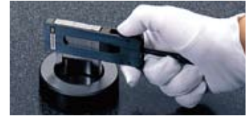
Gaging a bore using a pair of half round jaws and a holder
