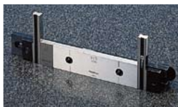
Use of B-type connectors in gage construction
