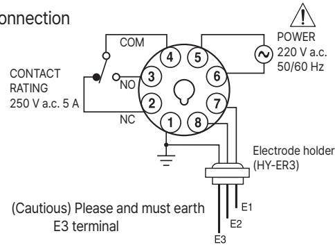
**Internal connection****① High sensitivity**
