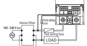
• In case of low voltage model, we suggest connect it as following picture. (90/110/130/160/200 A have fuse).
