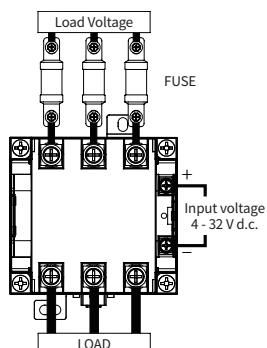
Fuse is not installed inside this product. We suggest you to use fast-acting fuse outside separately like the picture.
