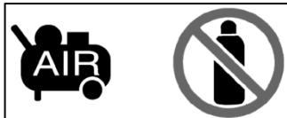
As this tool is designed and manufactured to operate using air pressure that is generated by an air compressor authorized by a safety certification authority, you cannot use any kind of gas—combustible gases such as oxygen and acetylene—except this. Otherwise, it may not only cause mechanical trouble but also malfunction or explosion, resulting in infliction of fatal injury on a user or those around him or her.
