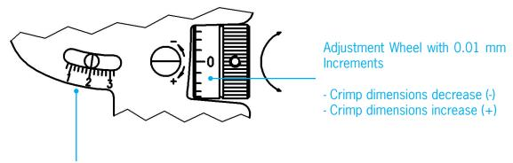
Scale with 1 mm and 0.2 mm Increments
