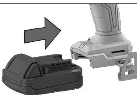
Remove the battery pack before starting any work on the product.
