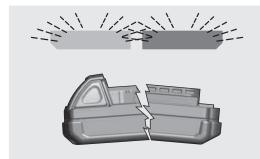
Continuous red: Charging Continuous green: Charging is complete Flashing red: Battery is too hot/cold Flashing red/green: Damaged or faulty battery pack
