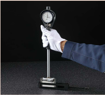
Setting a bore gage using a holder with a pair of Type I half-round jaws arranged as flat contact surfaces
