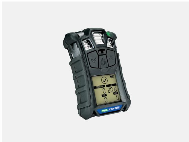
To help users confirm that a bump test was done, the MSA ALTAIR family of gas detectors uniquely shows a Bump Test checkmark on their display for 24 hours after a successful bump test. A bump test quickly confirms whether the gas entries are free, and if your sensor is functioning.
