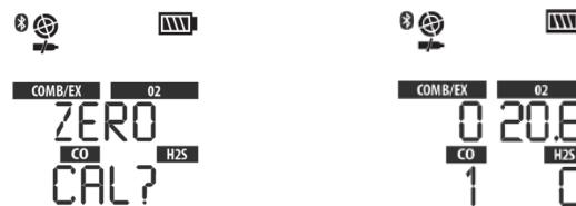
3. With the device exposed to fresh air, press the **⊕** button to confirm the **ZERO CAL?** screen. A sensor refresh and Zero Calibration will occur.
