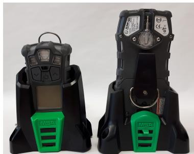
Insert the gas detector tightly into the charger as shown.
