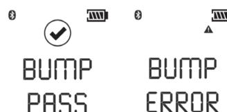
The **✓** symbol will be displayed in the Normal Operation mode and the Bump LED will flash green for 24 hours after a successful Bump Test.
