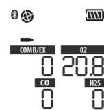
After the Bump Test completes, the device momentarily displays “BUMP PASS” or “BUMP ERROR” along with the label of any sensor that failed before returning to Normal Operation mode. If the device fails the Bump Test, perform a calibration as described in [4.10.2 Attach the Calibration Cap](#).
