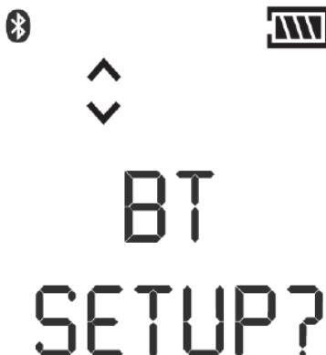
1. Press the ▲ button to enable or disable the Bluetooth communications device (ON/OFF).
