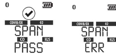
If a sensor is nearing its end of life, this "SPAN PASS" indication will be followed by the end of sensor life warning (♥ symbol). The ♥ symbol, and the gas type of the sensor nearing its end of life, will blink for 15 seconds when the device returns to Normal Operation mode. When in Normal Operation mode, the ♥ symbol is continuously displayed.
