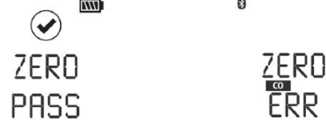
**i** During zero calibration the O<sub>2</sub> sensor is also span calibrated to 20.8% O<sub>2</sub> fresh air, adjusting the calibration curve as needed. During span calibration, the O<sub>2</sub> sensor's accuracy is checked against a known oxygen gas concentration without adjusting the calibration curve.
