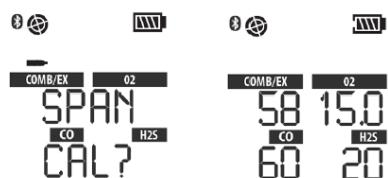
6. Press the button to calibrate (span) the device.
