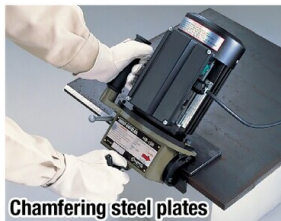
Chamfering steel plates
