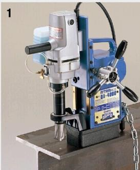
Align the pilot pin with the center punch mark of the hole to be drilled. Attach the machine to the beam with the proper safety chain and engage the magnet. Lower the drill down from the top limit switch location to the point of the pilot pin making contact with the material and engage the motor.
