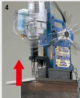
After the hole is completed, the QA Series machines will quickly return and stop at the top of the stroke, ready for the next hole.
