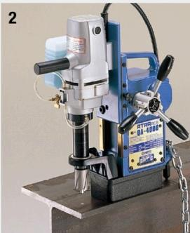
Engage the clutch by pushing the handles in towards the drill and the motor will begin feeding automatically.
