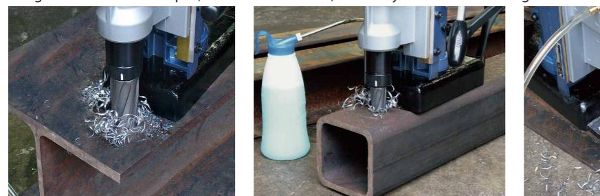
Portable Magnetic Base Drilling Machine
