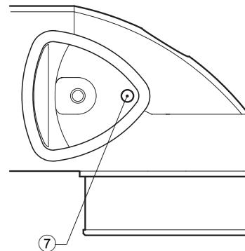
**3** Perform a trial run and wipe off extra grease that seeps out
